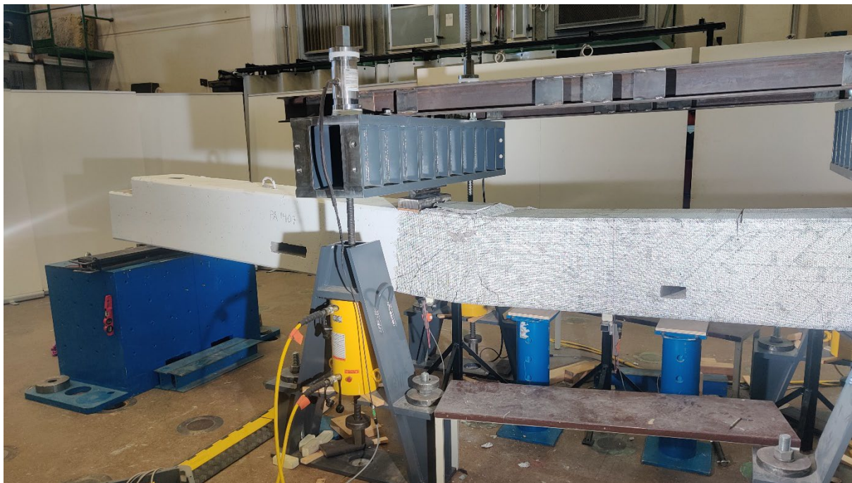
Figure 12. Full-scale testing of a beam. Photo © TAU/Aapo Räsänen.
