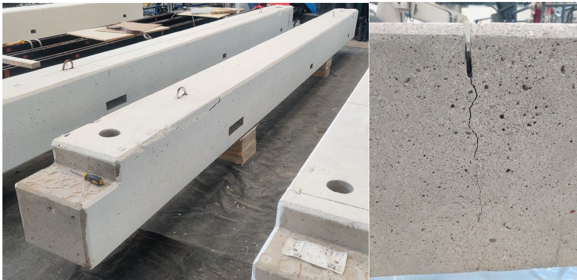
Figure 9. Support points too close to the midspan (left) and a crack on top of beam caused by this in conjunction with insufficient (inadvertently sawn) reinforcement (right). Photos © TAU/Aapo Räsänen.
